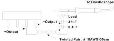
47uF and 0.1uF capacitor of proper polarity and voltage rating. The oscilloscope probe ground led should connect right to the ground ring of the probe and be as short as possible. The oscilloscope bandwidth should be at 20MHz and connected
