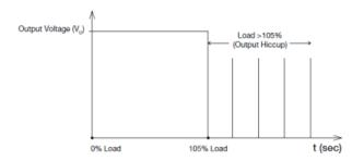
Additionally, if the  $I_0$  is <250% but >110% for a prolong period of time (depending on the load), the Over Temperature Protection (OTP) will be activated due to high temperature on critical components. The power supply will then go into hiccup mode until the fault is removed; and, the input voltage is removed, then reapplied.
