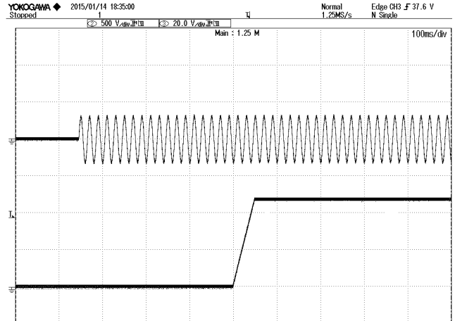
Figure 6: Vout start up with Enable on at 220Vac, 7.5A lout, TOP: Vin, 500V/div, 100mS/div BOTTOM: VOUT, 20V/div, 100mS/div
